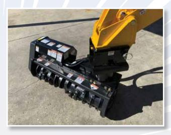
50in Fecon Mulching Head with optional 180 Degree Rotate
