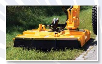
50in & 60in Rotary Deck with optional 90 Degree Swivel
