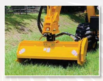
62in Standard Flail with optional 180 Degree Rotate
